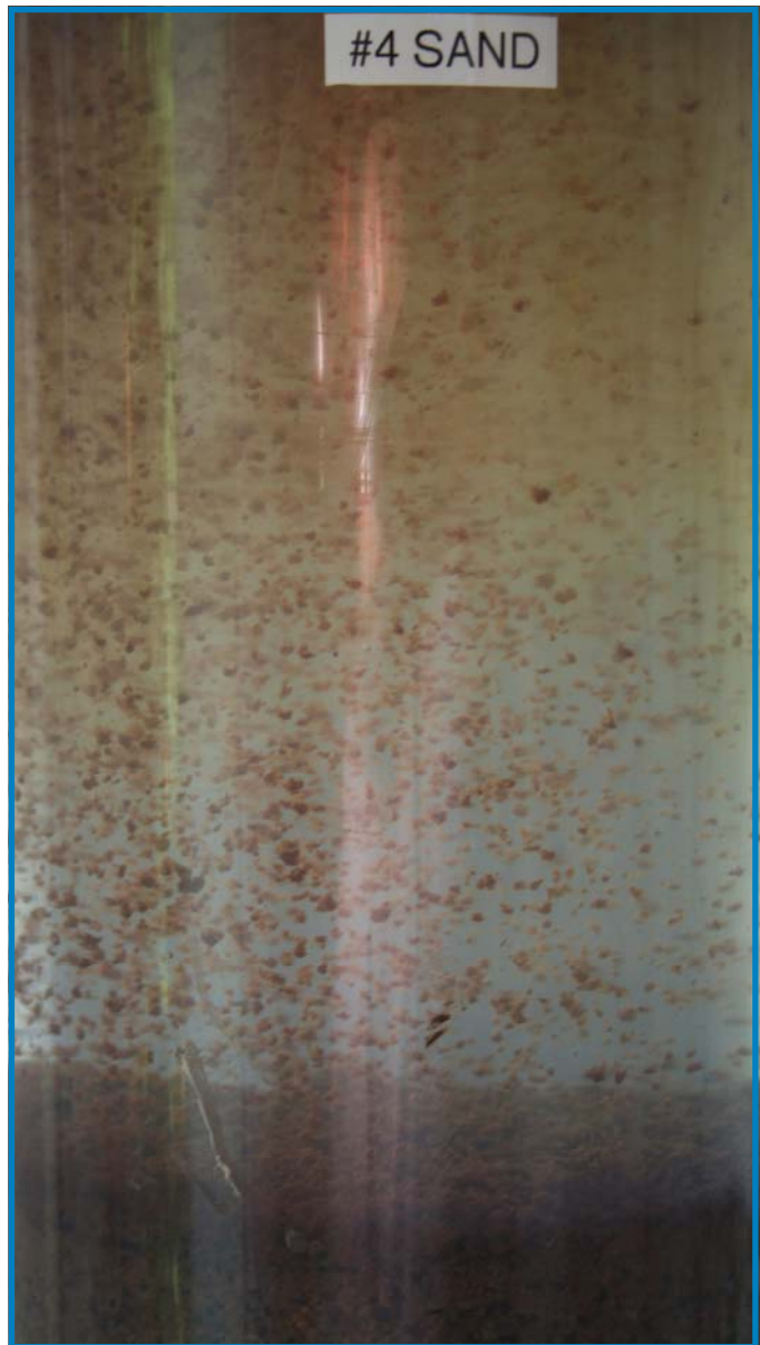
Rising floc from backwashing biological iron filter
